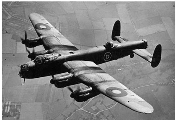
AVRO Lancaster Heavy Bomber. First utilised by Bomber Command in 1942. Designed with an unobstructed bomb bay, it carried bombs up to 10,000 kg. It had the largest payload of any aircraft of WWII. Powered by 4 Rolls Royce merlin engines, it was originally designed for daylight mission but became invaluable as a night bomber. After the war, a civilian version of the aircraft, the Lancastrian, was the first aircraft to take off on a transatlantic flight from the new Airport at Heathrow
